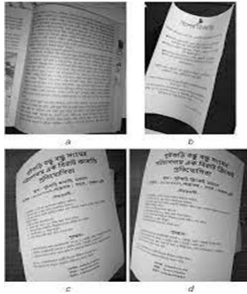
FIGURE 3. Geometric distortions of the images entered to the proposed OCR model
